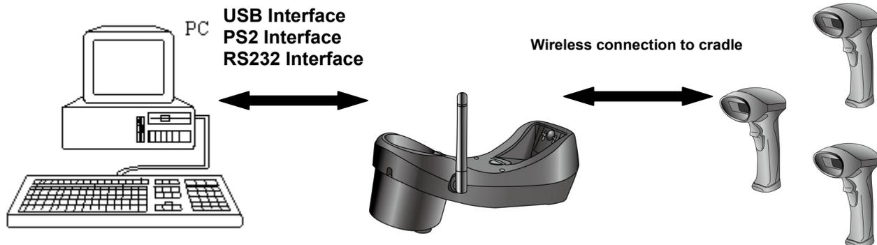
If multiple scanners are connected to the Host PC, in cradle-less mode, the data will be mixed up (simultaneous scan).
