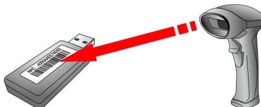
7. When being successfully connected to the dongle, the scanner will beep shortly one time with a high tone.
