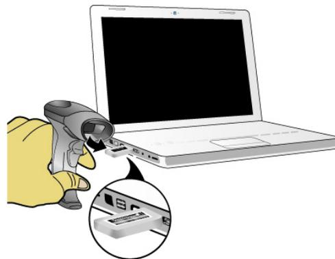
4. When being successfully connected to the dongle, the scanner will beep shortly one time with a high tone.
